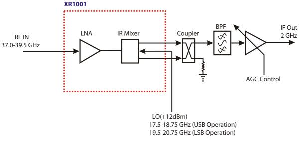
Mimix Broadband MMIC-based 33.0-40.0 GHz Receiver Block Diagram
